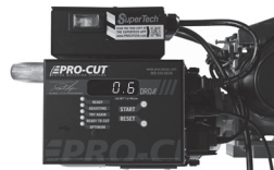
DRO computer compensated for lateral run-out to 0.0006" and ready to cut.
