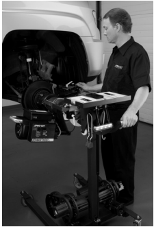
STEP 4. Technician sets cut depth.
