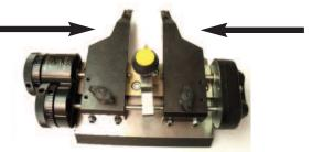
When adjusting the gib screws on the back of the arms, do not allow the "point" of the 7mm jam nut to come in contact with the tool holder plate. The flat part of the nut, not the point, should be facing down. (See picture below, left.)
