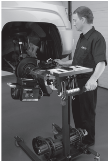
STEP 4. Technician sets cut depth.
