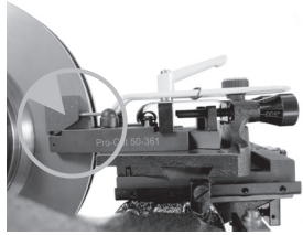
The chip deflector rides over the cutting arms as shown above.
