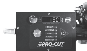
DRO computer in READY mode displaying speed.
