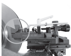
The chip deflectors ride over the cutting arms as shown above.
