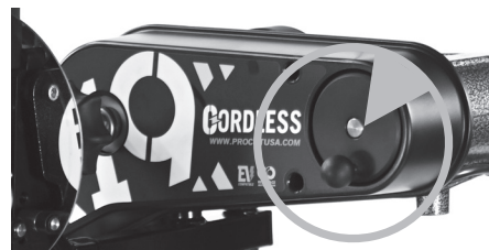
Move the cutting head by turning the clutch knob shown above, clockwise for away from the rotor, counter-clockwise for towards the rotor.
