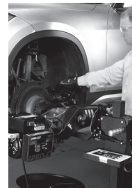
STEP 4. Technician sets cut depth.
